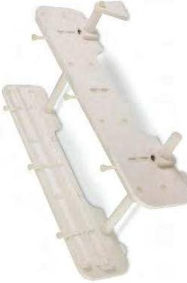
A wide range of interchangeable comb and spacer options allows a large number of techniques to be easily accomplished including: DNA Sequencing, 2-D analysis, Micro-satellite analysis, DNA fingerprinting, Gel shift assays, Single-Strand Conformation Polymorphism (SSCP), Heteroduplex and Oligonucleotide analysis.
