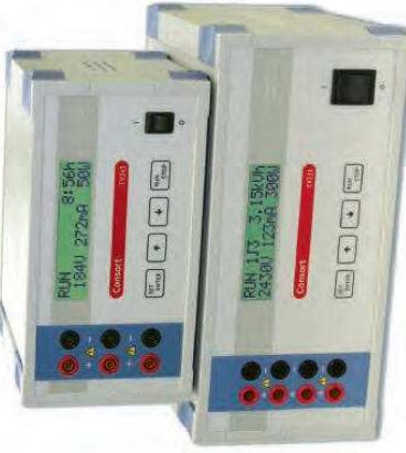
The Consort Mini EV245 power supply is ideally suited for use with small electrophoresis systems. It occupies little space within the laboratory, is portable and has several other features:-
