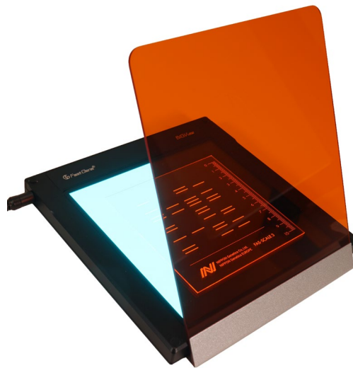
Figure 3: FastGene® Slim Blue Green View LED Transilluminator in use example with amber filter shield and fluorescent gel card.
